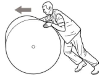
Churning (loads are moved by pivoting/rolling along the base edges)
