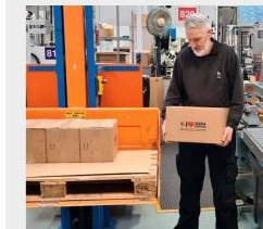
→ Photo 3 Operator lifts roll from press and boxes at same height
